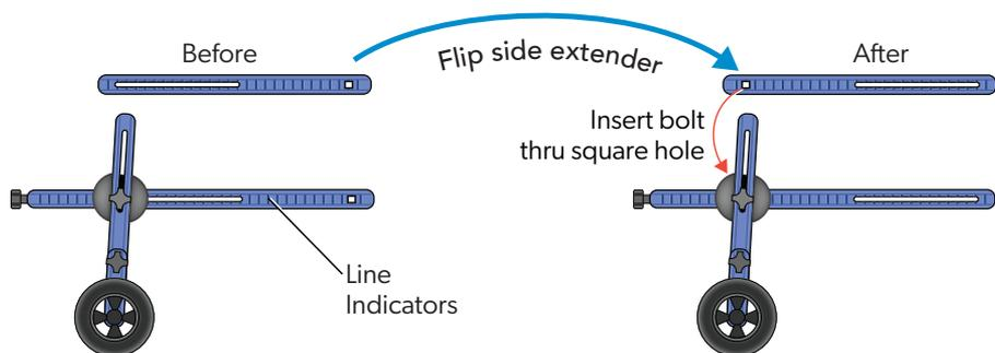
6. Insert the bolt through the middle square hole on the frame and through the side extender square hole.
